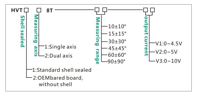
E.g : HVT 128T-10-V2 : standard/Dual axis/ $\pm 10^{\circ}$  Measuring range /  $0\sim 5V$  output Voltage
