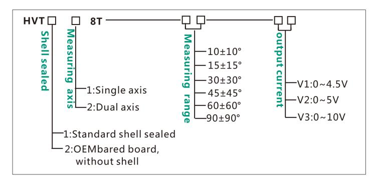
E.g : HVT 12 8 T -10-V2 : standard/Dual axis/ $\pm 10^\circ$  Measuring range /  $0 \sim 5$  V output Voltage
