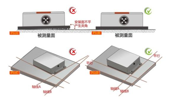
The mounting surface of the sensor must be tight, flat and stable when it is fixed to the surface to be measured.
