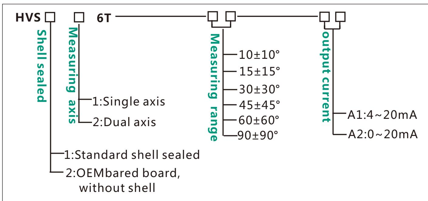
E.g : HVS 12 6 T -10-A1 : standard/Dual axis/ $\pm 10^\circ$  Measuring range /4mA-20mA output current
