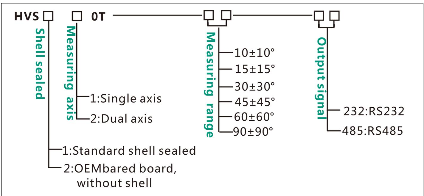
E.g : HVS 12 0 T -10-232 : standard/ dual axis/±10° Measuring range /RS232 output
