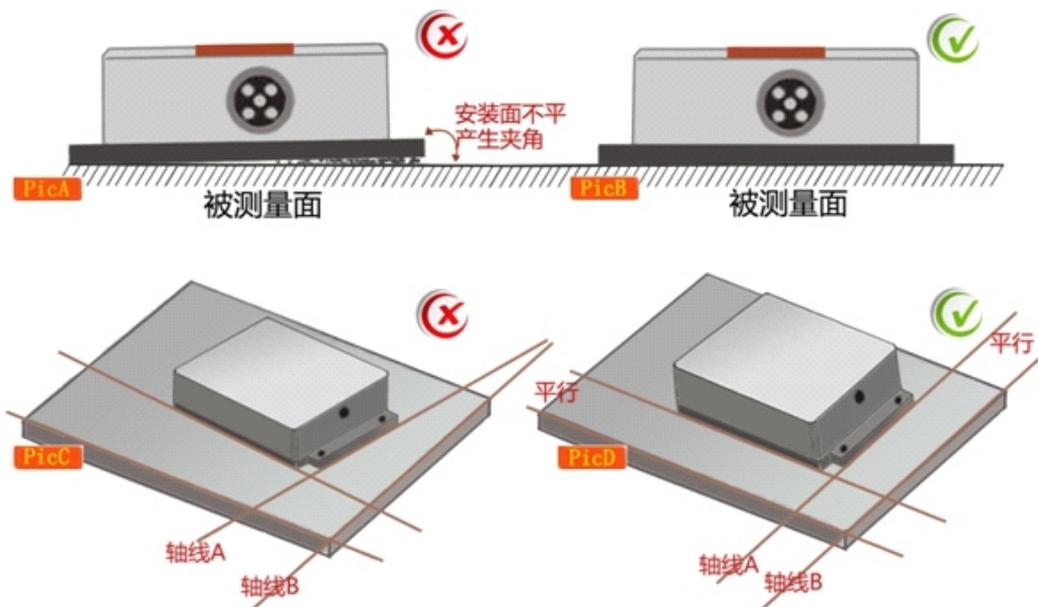
The mounting surface of the sensor must be tight, flat and stable when it is fixed to the surface to be measured.
