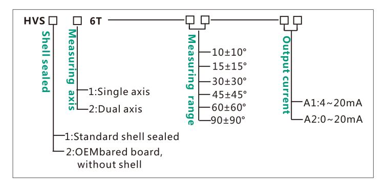
E.g : HVS  $\bf 11$  6 T - $\bf 10$ - $\bf A1$  : standard/single axis/ $\pm 10^\circ$  Measuring range /4mA-20mA output current
