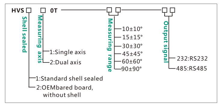
E.g: HVS 110 T-10-232: standard/Single axis/±10° Measuring range /RS232 output
