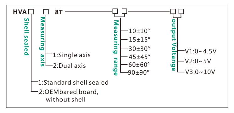
E.g : HVA 128T-10-V2 : standard/Dual axis/ $\pm 10^{\circ}$  Measuring range /  $0\sim 5V$  output Voltage
