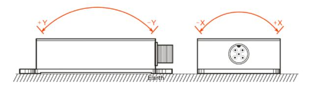
The axis of the sensor must be parallel to the axis to be measured, and the two axes should not be angled as much as possible.
