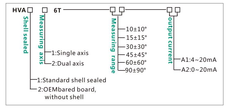
E.g : HVA 12 6 T -10-A1 : standard/single axis/±10° Measuring range /4mA-20mA output current
