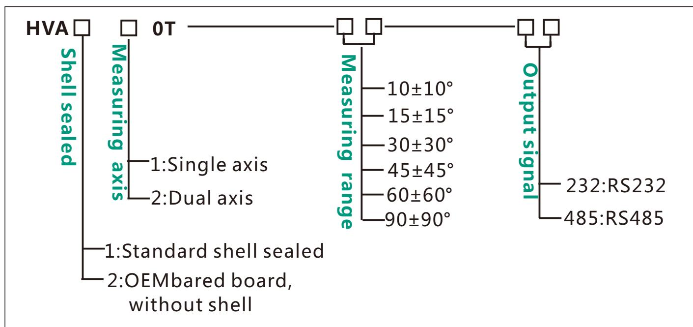
E.g : HVA 120 T - **10-232** : standard/ dual axis/ $\pm 10^\circ$  Measuring range /RS232 output
